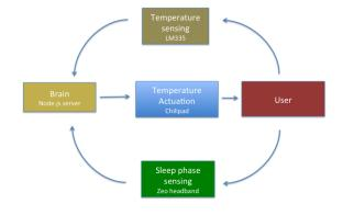
Figure 1: A simple diagram illustrating our current system. It illustrates the 4 major subsystems of our system, temperature actuation, temperature sensing, sleep phase sensing, and "brain".
